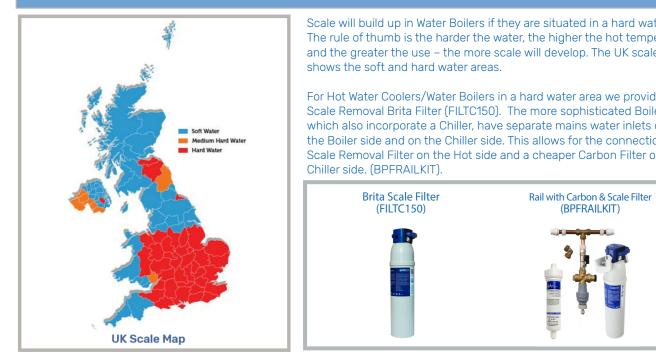
The Carbon Filter on mains connected Coolers should also be exchanged every six months. This is to avoid Bacteria "shedding" into the Cooler from Bacteria which over time can grow inside the filter.
